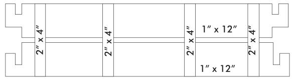
2.The inside of the panel (non 2" x 4" side) should be smooth, so sand as needed. Carriage bolts should be inserted with the smooth end *toward* the inside, with the nut and washer on the outside.
